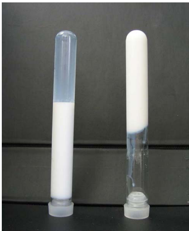
Fig. 1 Picture of gel formation of SLN after cooling, on the left after holding for 5 min at 5 °C, on the right after holding for 60 min at 5 °C
